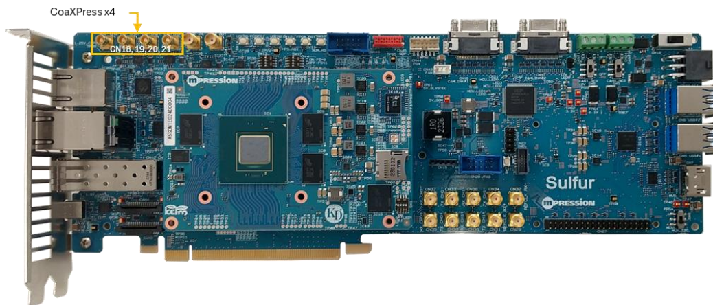
Figure 2-25 CoaXPress Connector Layout
